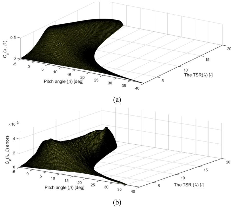
Fig. 4. The aerodynamic power coefficient  $C_p(\lambda, \beta)$  surface for: (a) original one; (b) model error.
