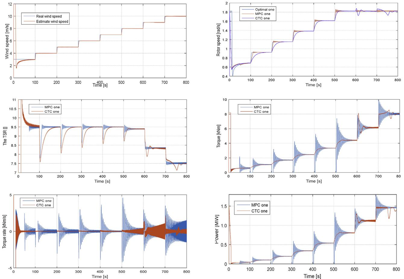
Fig. 2. Simulation results comparisons between the CTC and proposed torque control strategy.
