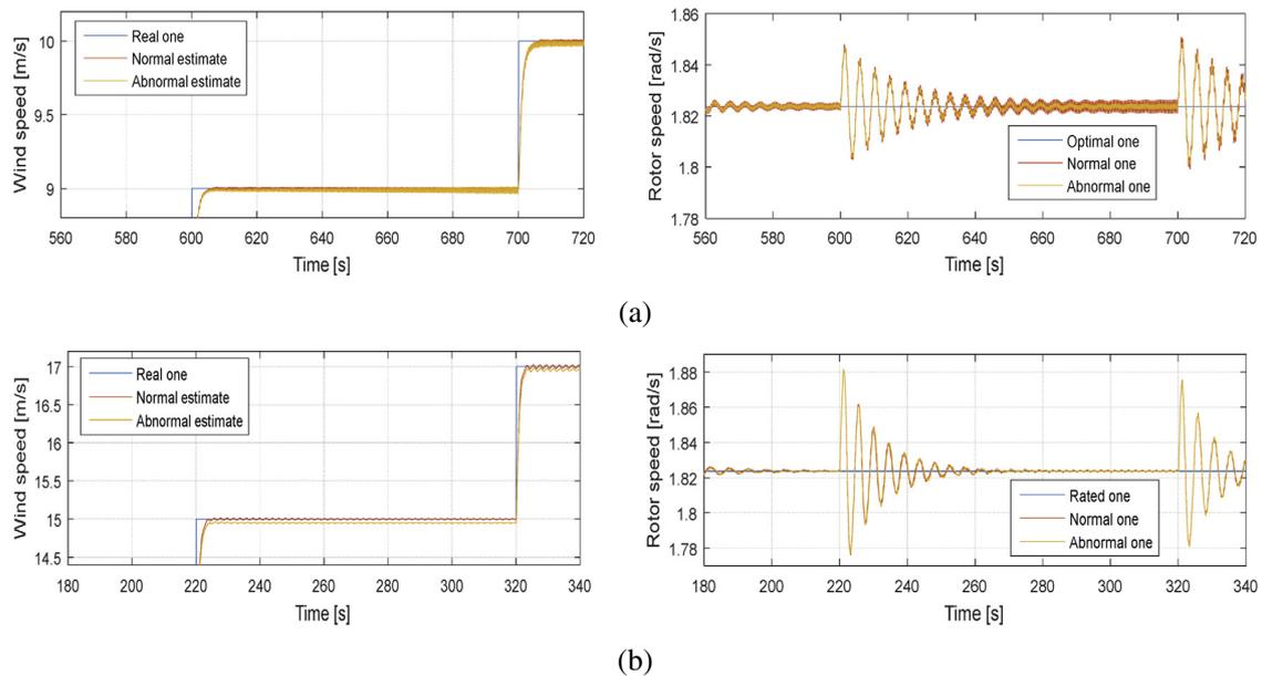
Fig. 5. Simulation results comparisons between normal case and abnormal case with model error under: (a) torque control strategy; (b) pitch control strategy.
