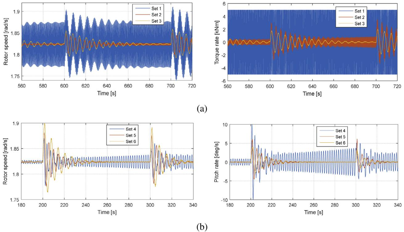
Fig. 6. Simulation results comparisons with different weighting factors under: (a) torque control strategy; (b) pitch control strategy.
