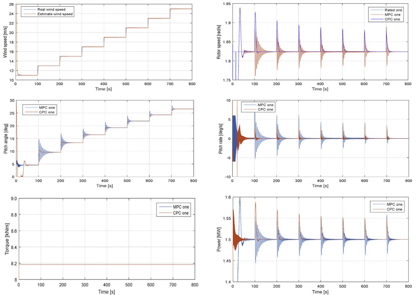
Fig. 3. Simulation results comparisons between the CPC and proposed pitch control strategy.
